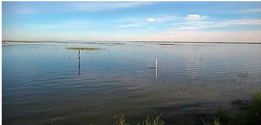
Fig. 2.8. Surveying rods to monitor the level of water in Lake Ribachye (June 2017)
